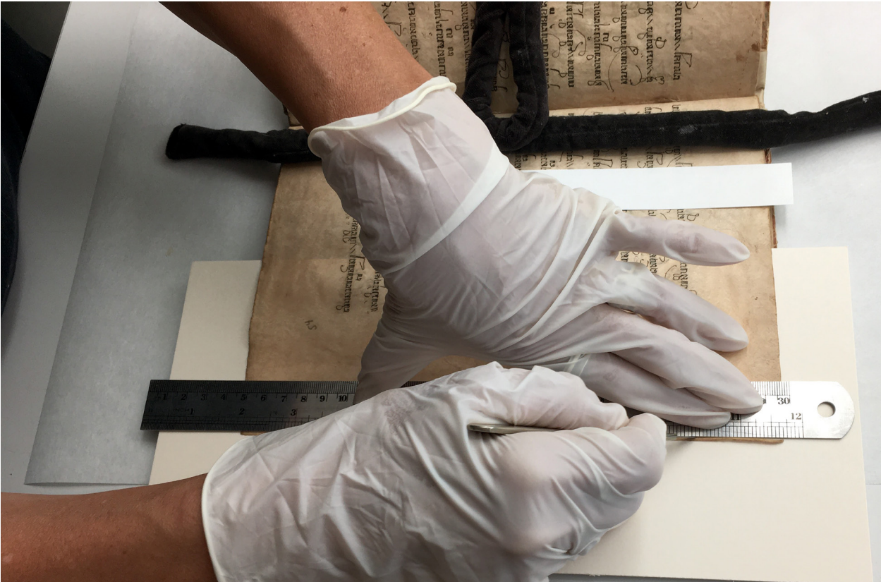
Fig. 2b: Or. 1928, extracting the sample of dluwang from the fore-edge of p. 54.
